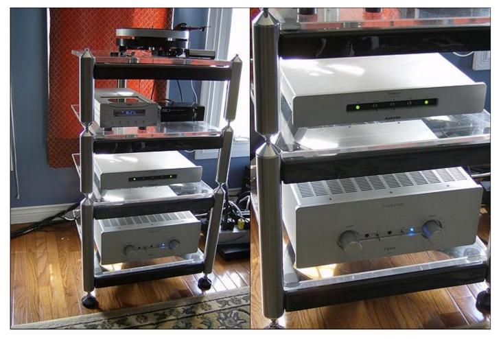
All of the Opéra Référence's 30 watts run in class A via a quartet of EL34 tubes. The input stage features a trio of NOS 5965s for phase splitting and driver duties. The amp sits on a trio of large nickel-plated brass cones and the chassis is aircraft-grade aluminum with a 10mm thick front panel. Available finishes include brushed aluminum or anodized black.
